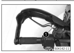
Adjust the basic position of the clutch lever to your hand size by turning adjusting wheel ①.
