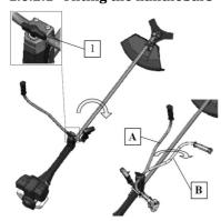
It is possible to tilt and turn the handlebars of your brush cutter/trimmer to a storage position for easier storing. The tilting procedure is described below.
