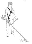
After the brush cutter/trimmer is started, hang it on the harness and grasp the handlebars properly.
