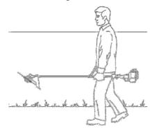
! The engine must always be off and the safety cover must be put on the cutting tool during transport.
