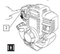
The procedure for the warm start is the same as for the cold start, except for the choke switching. The choke lever (2) has to stay in the lower position.
