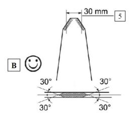
Perfect results of the cutting tool can only be ensured if the blades are properly sharpened. Slight sharpening can be done with a hand sharpening stone. For bigger blunting it is necessary to use a tool sharpener.
